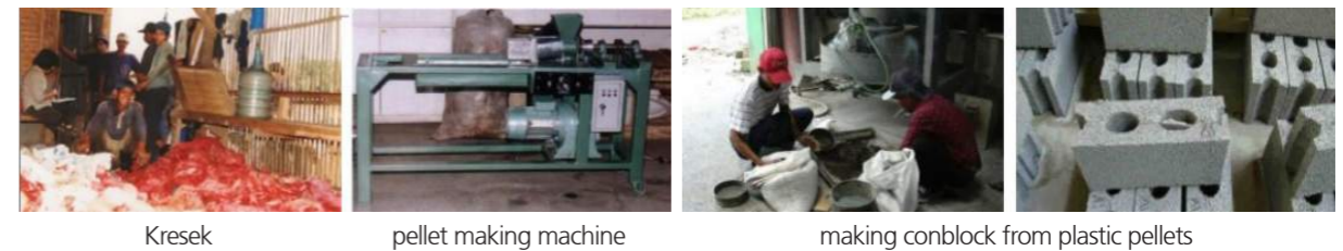
Figure 26 Recycle plastic bag waste into building materials (conblock)
